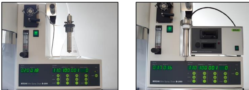
Figure 11: Spray drying nozzles used for the mini spray dryer in this work; two-fluid nozzle (left), ultrasonic nozzle (right)
